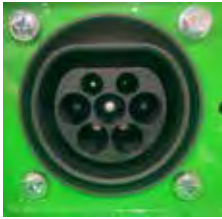
Standard Type 2 charging inlet on loader
