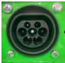
Standard Type 2 charging inlet on loader
