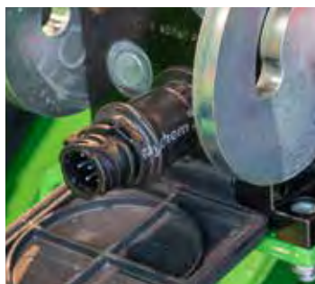
Adapter kabel for redskapets Multi connector A36679
